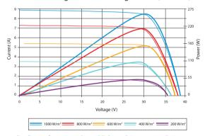
Excellent performance under weak light conditions: at an irradiation intensity of 200 W/m² (AM 1.5, 25 °C), **96.5%** or higher of the STC efficiency (1000 W/m<sup>2</sup>) is achieved
